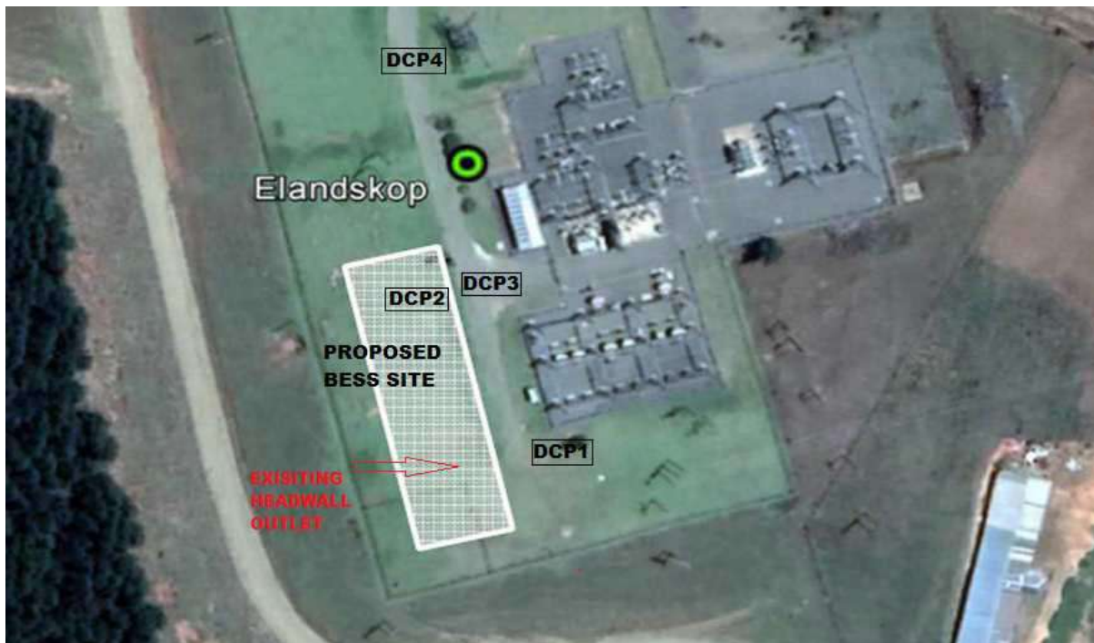
Figure 15: DCP Test Positions (Geotechnical Report, 2019)
